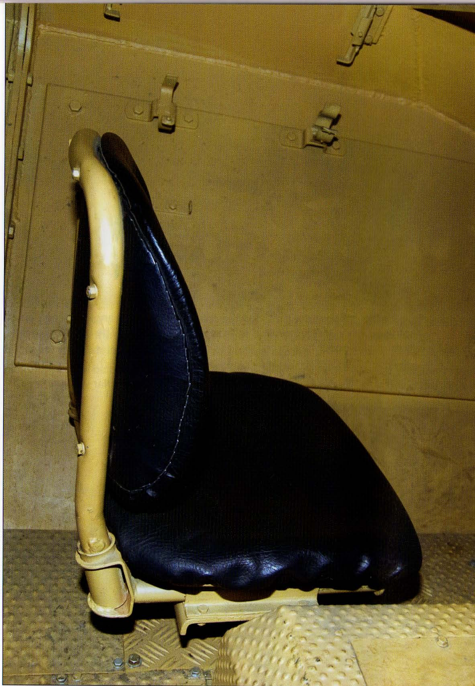
The driver's seat is covered in black leather. Leather color for seats varied by manufacturer. Sand or brown-red also were colors for the leather seats. Both seats have flip-up bases and could be removed. This vehicle used the same seats for the driver and the commander that were used in the German Panzerkampfwagen (tanks).
