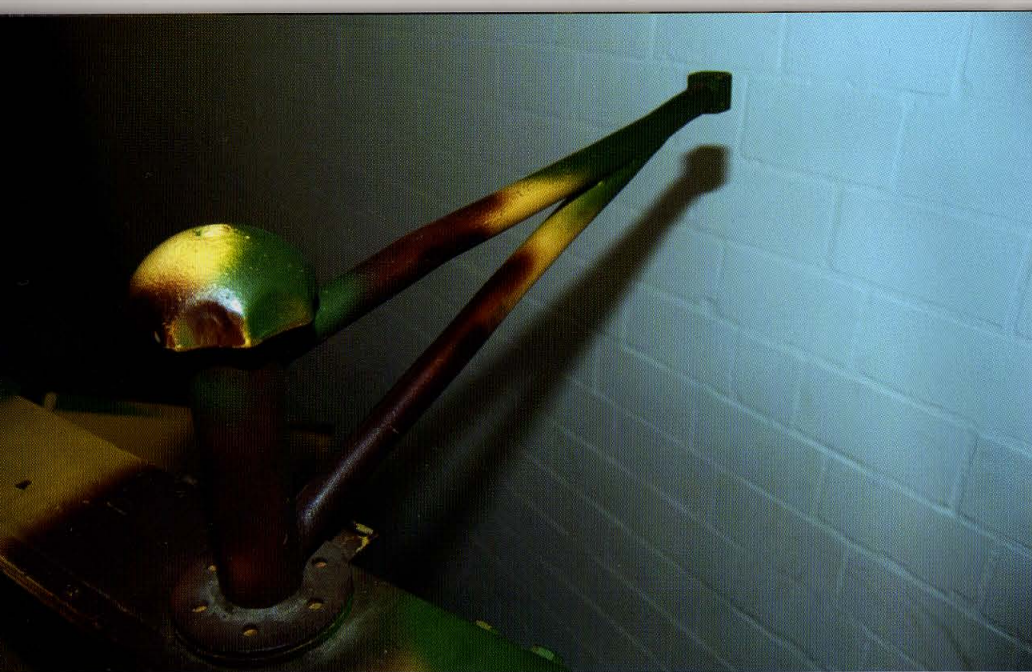
The pivoting machine gun mount is attached on the upper rear superstructure with a stud and accommodates an MG 34 or an MG 42 7.92 mm machine gun.
