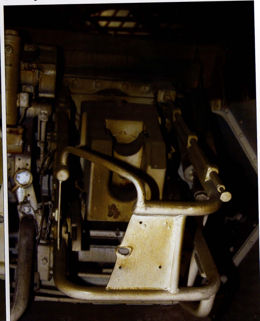
The recoil guard for the KwK 37 L/24 gun is right of the centerline in the crew compartment. The recoil guard was altered so the gunner was seated while loading the gun.
