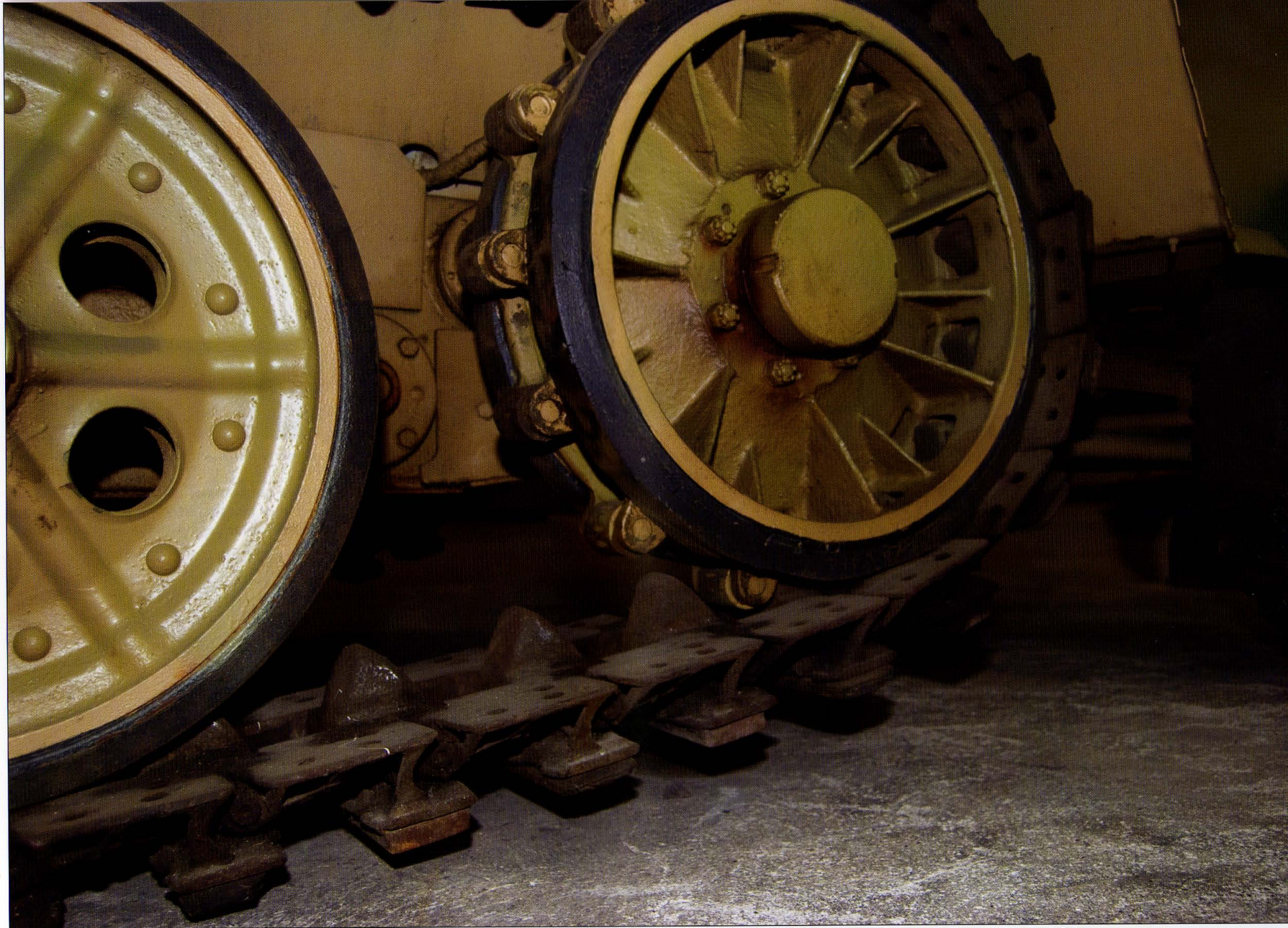
The right drive sprocket of this SdKfz 251 Ausf D is visible with the drive tooth on the inside of the track.
