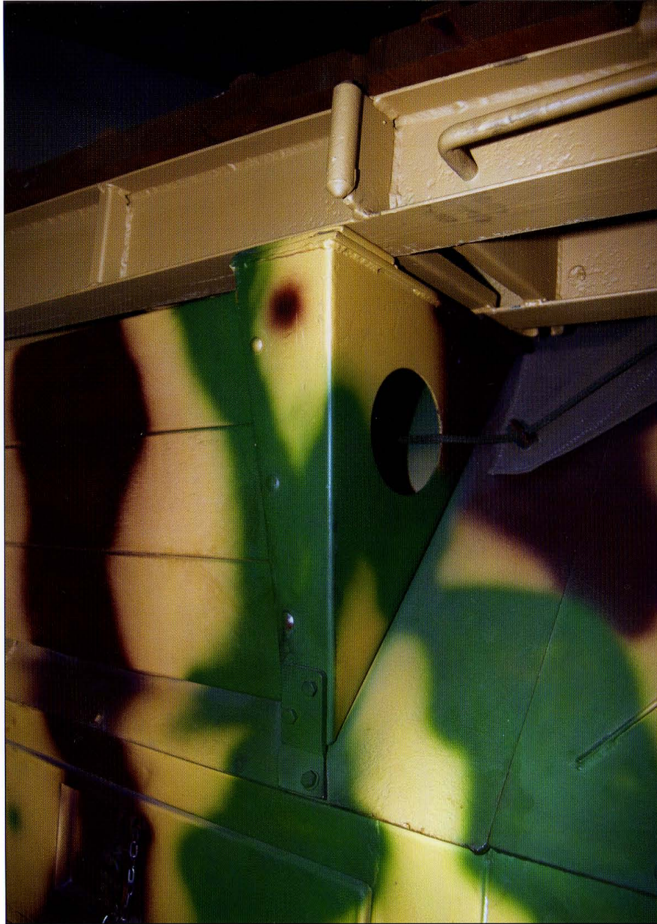
This view shows the right front support bracket of an SdKfz 251/7 Ausf D. The support brackets were bolted against the upper superstructure of the German half-track. The bracket's metal profiles were made from metal pieces that were welded together. All support brackets had a circular aperture in the front face. Atop the support bracket is a single Übergangsschiene 8.
