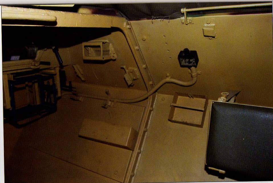
This view shows the right console. The armored superstructure had two sections bolted together behind the driving compartment. The bolts are visible here. The frame just in front of the leather-covered benches held spare armor glass blocks that could be inserted in the frame in front of the side slit. The cable attached on the inner armor plate connected the radio with the antenna socket, mounted on the edge of the upper superstructure. The antenna socket and antenna mast were only carried when a radio was built into the half-track.
