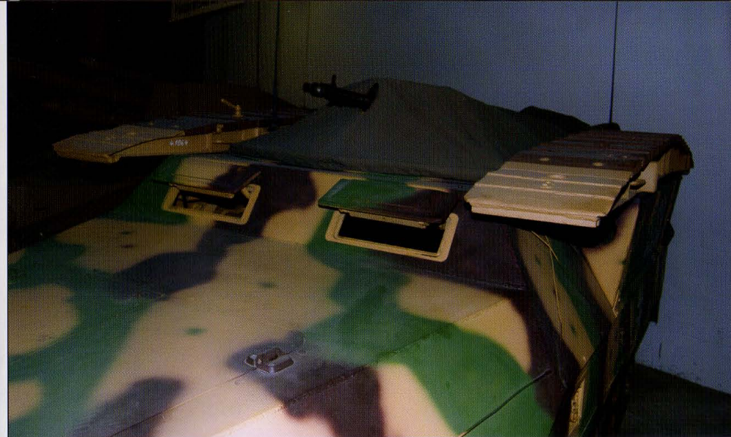
The two Übergangsschienen 8 were a typical feature of the SdKfz 251/7 Ausf Ds. No other variant of the SdKfz 251 was ever equipped with these kinds of assault bridges. The crew compartment as well as the armor shield for the MG 42 machine gun were covered with canvas. The overall height of the SdKfz 251/7 engineer vehicle was 2.70 meters, which was .95 meters taller than the standard SdKfz 251/1 troop carrier.
