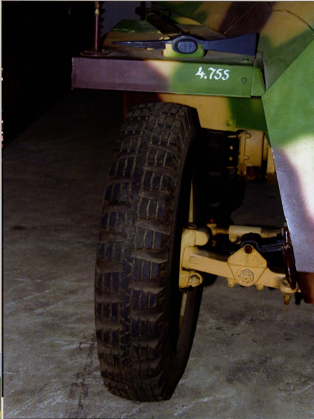
This view focuses on the right suspension unit, the straight, front fender—a common vehicle feature that made production faster—and the right-side front tire. The Ausf D had a 32 cm ground clearance and a 12.5 meter turning radius.
