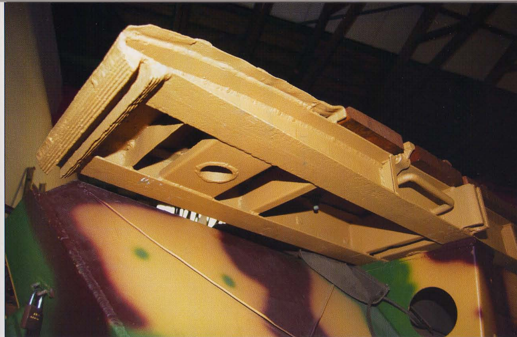
The rear lower surface of the right assault bridge has a welded-on handle so the crew can carry the bridge.
