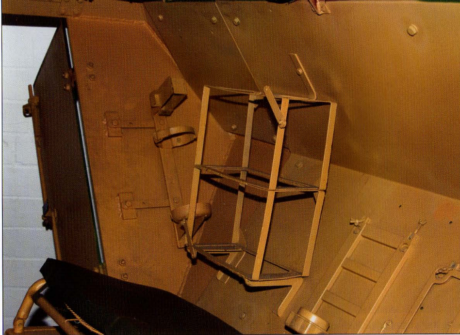
The rectangular frame, located on the rear cabin compartment, was a unique feature for the SdKfz 251/7 Ausf D.
