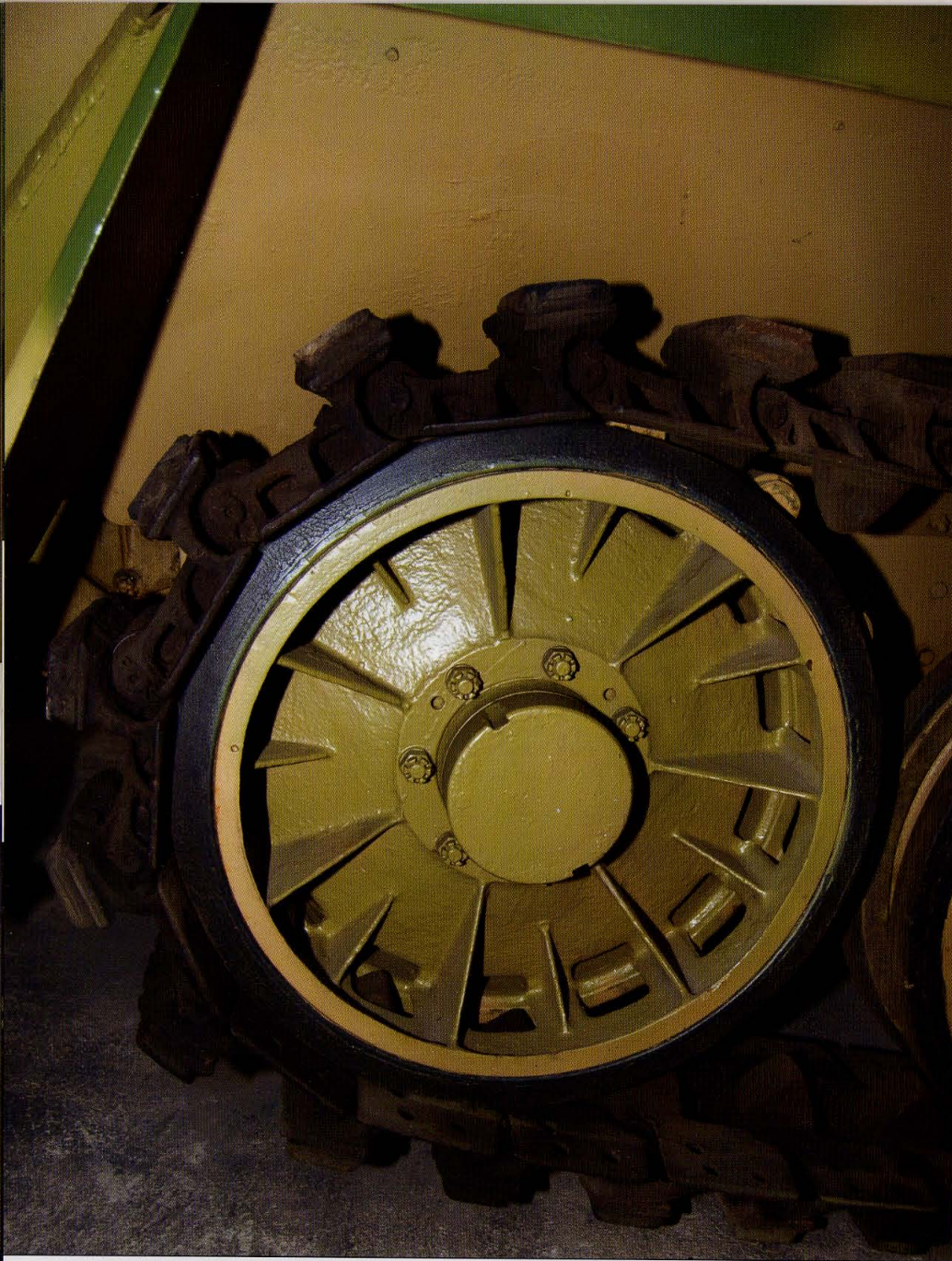
Protected by a front fender, left drive sprockets of early and standard production SdKfz 251 Ausf Ds had a flat-surface cover cap with two notches. These notches were removed on late production SdKfz 251s, and the cover cap was changed to a rounded-surface with three rectangular metal sheets welded on its side.
