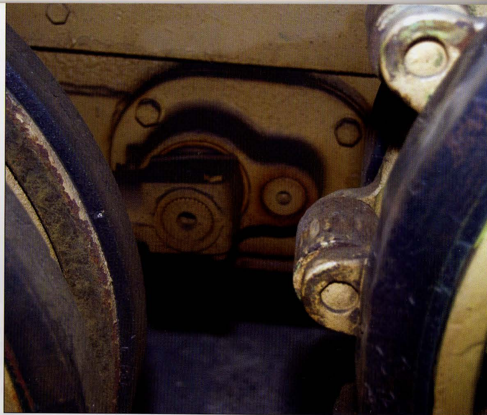
The wheel suspension arm was attached to the H kl 6p chassis frame. This device connected with the first twin wheel, which was behind the right drive sprocket.
