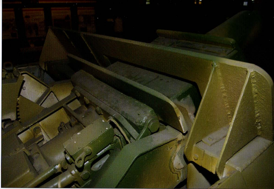
This view shows the upper part of the KwK 37 L/24 gun with the armor shield on the rear. The armor shield was welded to the vehicle superstructure, and a smaller shield was mounted on the gun barrel. Note the two triangular gussets on the shield's right side.
