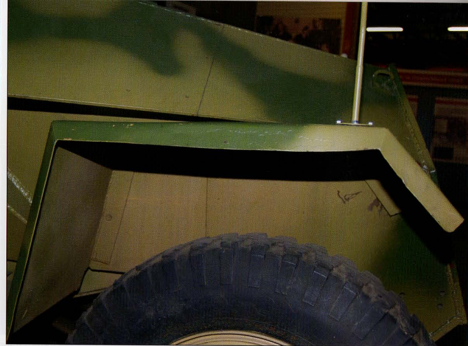
This rare, front-bent right fender indicates an early production SdKfz 251 Ausf D.
