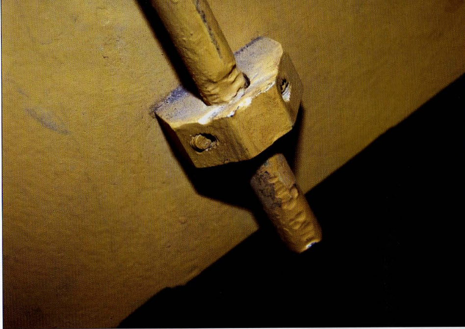
The rod's U-shaped guide was attached to the lower, inner surface of the armored rear door on both the left and right doors.
