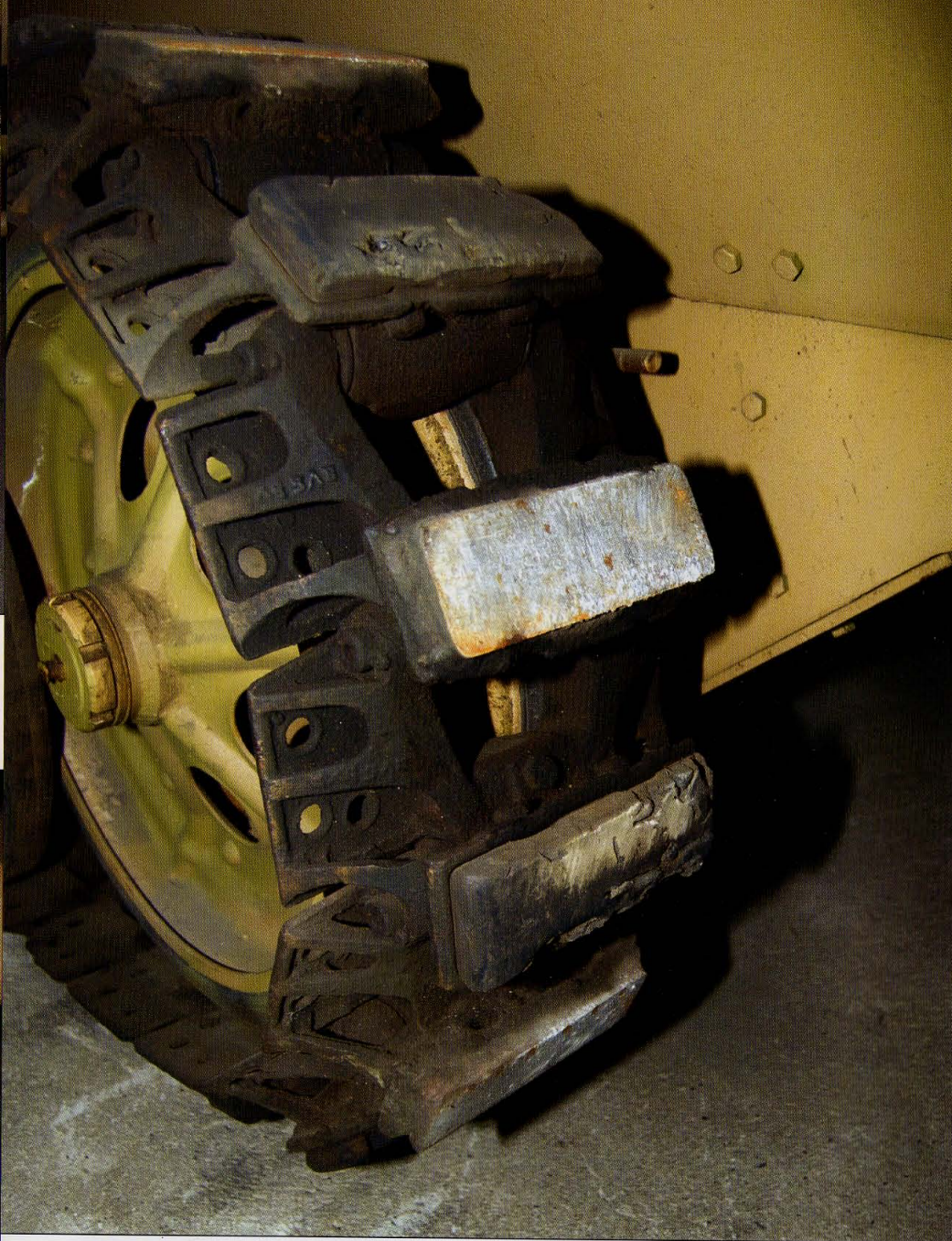
This view shows the left idler of an early production SdKfz 251 Ausf D. These tracks were equipped with steel caps, which reduced the vehicle's top speed to 30 km/h. At higher speeds, the steel shoes often vibrated loose and got lost. Most Ausf D tracks were equipped with rubber pads rather than steel pads.
