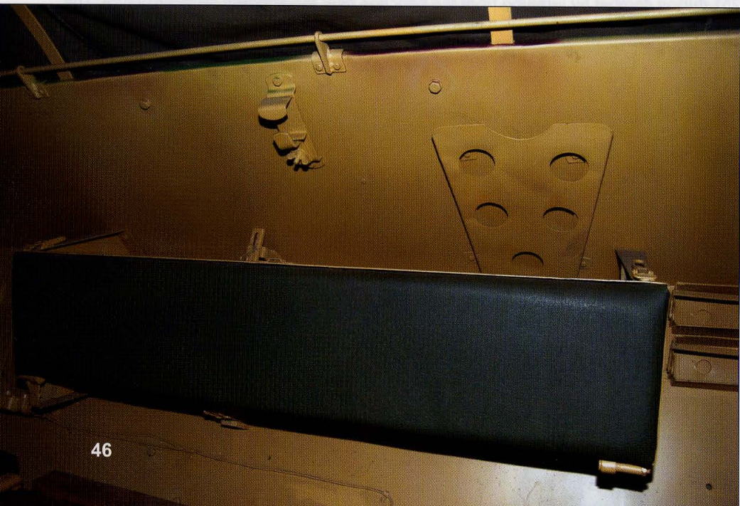
The holder, in the center right of this photo, is attached to the rear inner armor and housed a fire extinguisher. The fire extinguisher is not mounted on this SdKfz 251/7. Usually, the fire extinguisher was secured in its holder with a leather belt. The fire extinguisher holder was attached only on the left side of the vehicle. The position of the fire extinguisher is unique for the SdKfz 251/7 pioneer vehicle. The standard SdKfz 251/1 troop carrier had the fire extinguisher mounted on the right rear armor plate. The Ausf D and Ausf C were the only versions equipped with a fire extinguisher in the crew compartment. Earlier vehicle versions had the fire extinguisher placed on the vehicle's outer superstructure.
