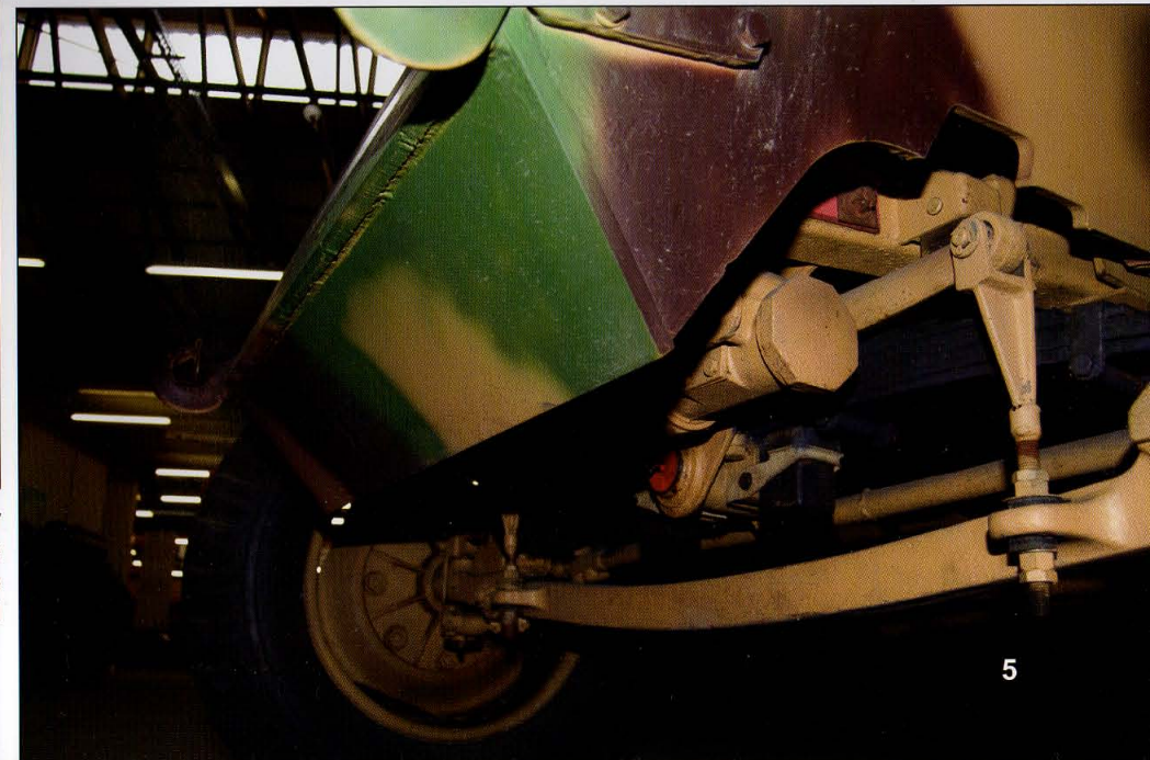
The small, lower armor plates protected the steering arm and the lower part of the radiator, which was cooled by two fans.
