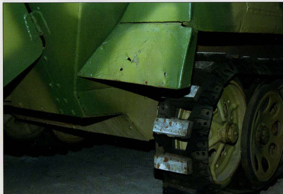
The right rear fender on an early production Ausf D was welded on the rear lower superstructure. The vehicle had a much steeper angle on the rear fender than previous versions of the half-track. The license number was painted on the left fender only. Only a few vehicles had license numbers painted on the right rear fender as well.
