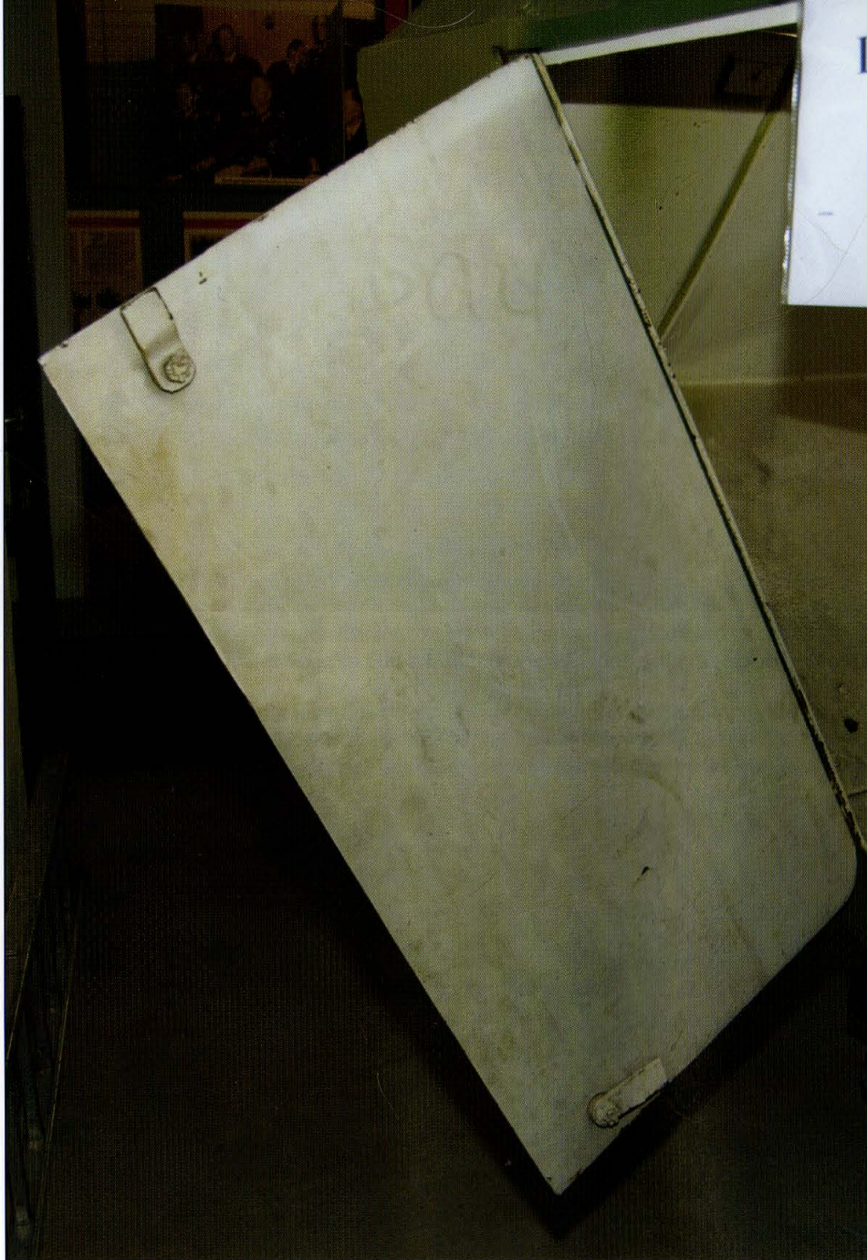
Early production German half-track vehicles lacked the rod-shaped opening mechanism that was a typical feature on standard production Ausf Ds. The rear doors could not be opened from inside, which made exiting through the rear doors impossible.
