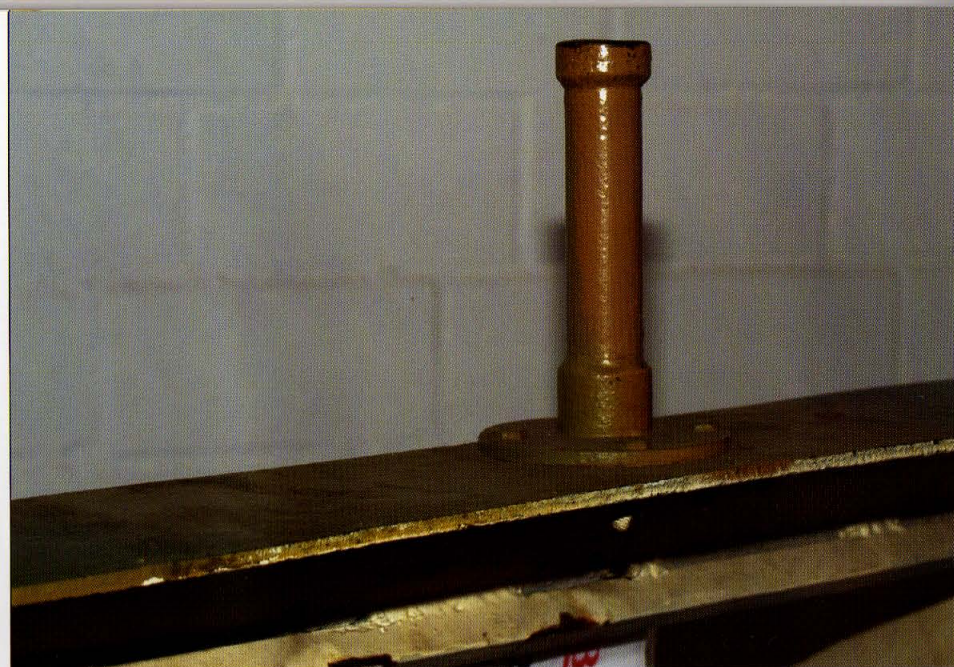
The pivoting machine gun mount was attached on a pin. Bolts secured the pin to the upper superstructure's connecting frame. The mount could be removed from the pin, and a number of crews removed the device when the machine gun was not mounted.
