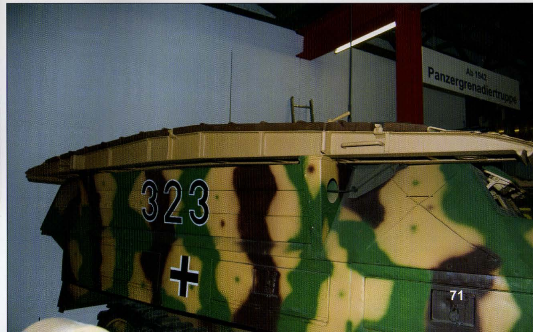
The space between the two support brackets is filled with a wooden planking. A number of SdKfz 251/7s had this planking, but the main part of the engineer variant lacked of the wooden planking on the upper superstructure.
