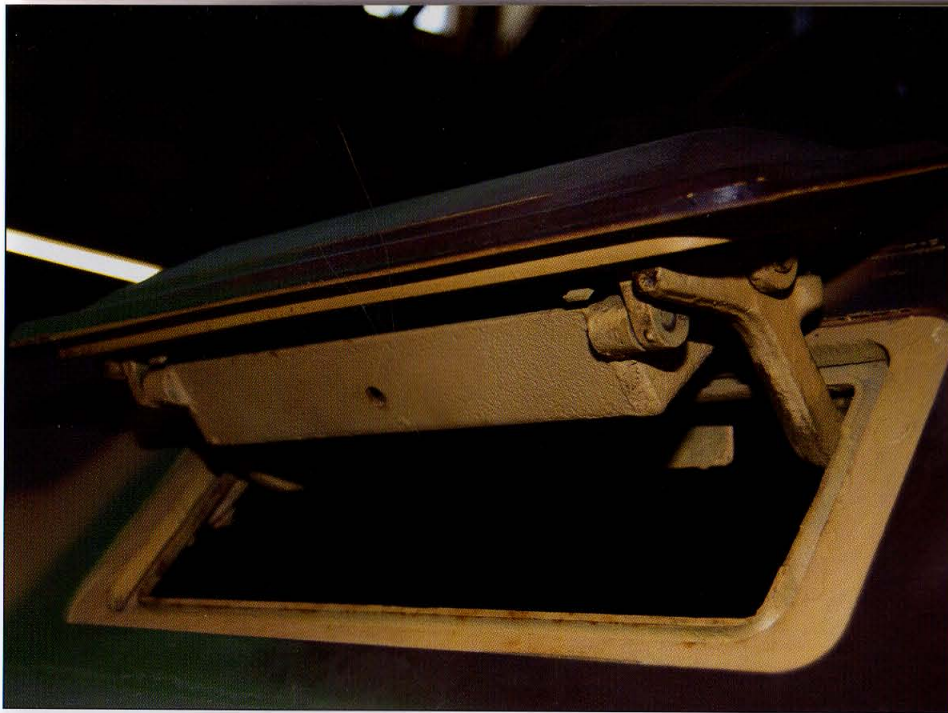
This retractable armor plate is on the left front vision port of an Ausf D. The armor shield was opened and retracted manually by a lever located inside the crew compartment.
