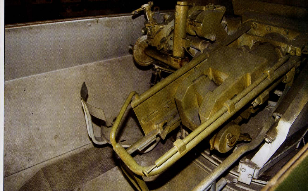
This view shows the left side of the recoil guard for the KwK 37 L/24 gun. The gun's breech mechanism is visible. The 7.5 cm gun allowed the SdKfz 251/9 to engage enemy strong points, but its weak armor made the half-track less suited to a role as a tank destroyer despite its ability to fire armor piercing shells.
