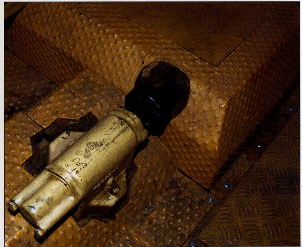
The gear-shift gearbox was located on the right, behind the fairing for the gearbox.
