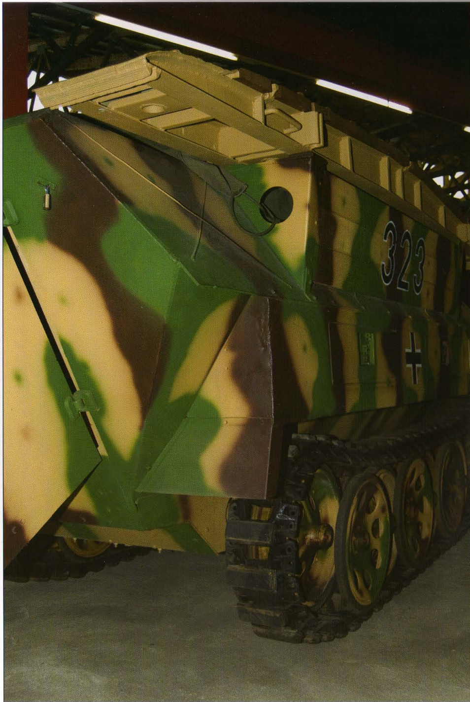
The rear arrangement of the right Übergangsschiene 8 rests on the support bracket. Note the circular aperture is located on the rear bracket.
