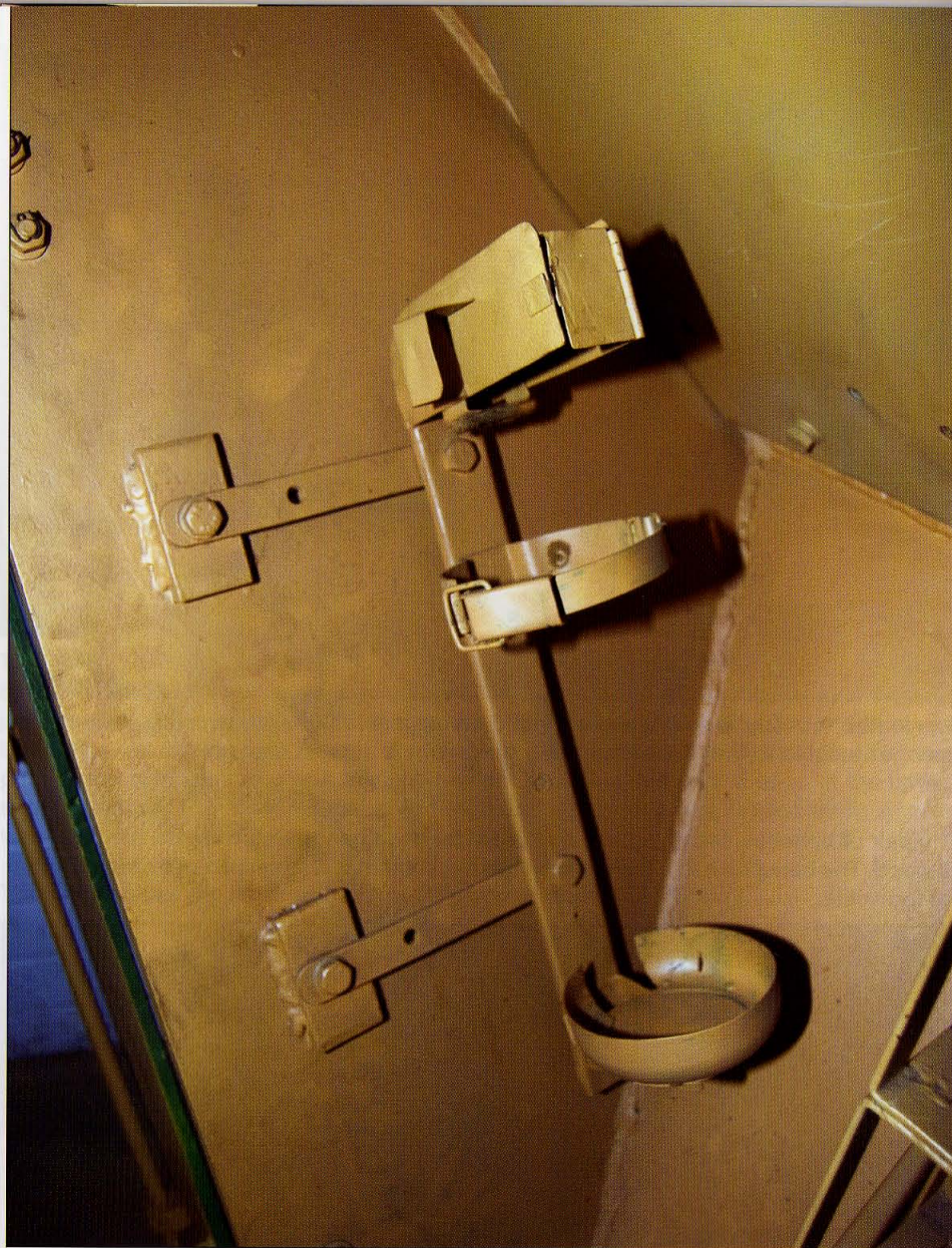
The holder, in the center right of this photo, is attached to the rear inner armor and housed a fire extinguisher. The fire extinguisher is not mounted on this SdKfz 251/7. Usually, the fire extinguisher was secured in its holder with a leather belt. The fire extinguisher holder was attached only on the left side of the vehicle. The position of the fire extinguisher is unique for the SdKfz 251/7 pioneer vehicle. The standard SdKfz 251/1 troop carrier had the fire extinguisher mounted on the right rear armor plate. The Ausf D and Ausf C were the only versions equipped with a fire extinguisher in the crew compartment. Earlier vehicle versions had the fire extinguisher placed on the vehicle's outer superstructure.
