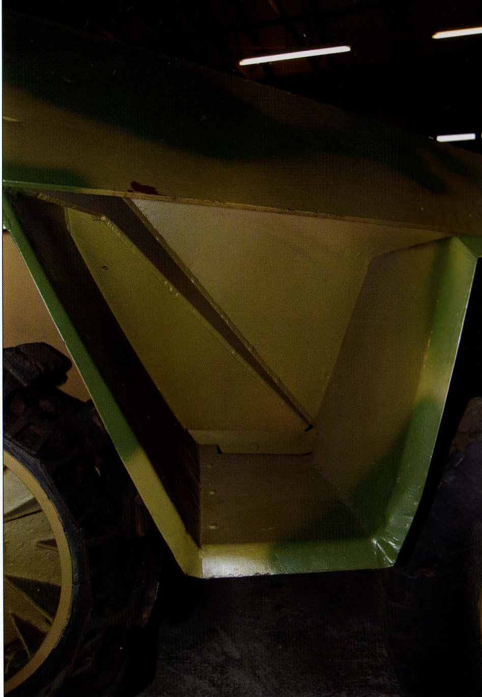
As stated previously, very early production Ausf Ds used the Ausf C's front fender design. These early vehicles had shorter plates connecting the front fender with the track fender. The armor body's slanted fairing also was different from standard production models.
