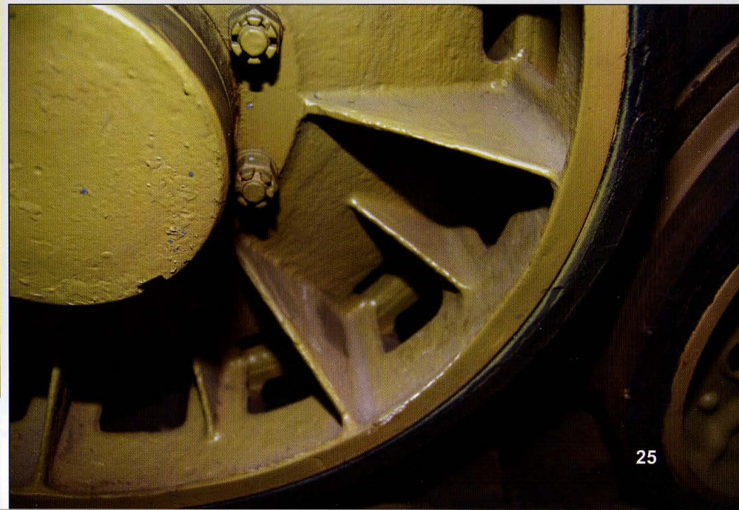
This view shows the spoke-shaped extensions of the left drive sprocket. Like the other wheels on the tracked suspension, the drive wheel was equipped with a rubber tire.
