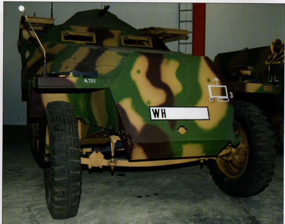
This rare, front-bent right fender indicates an early production SdKfz 251 Ausf D.
