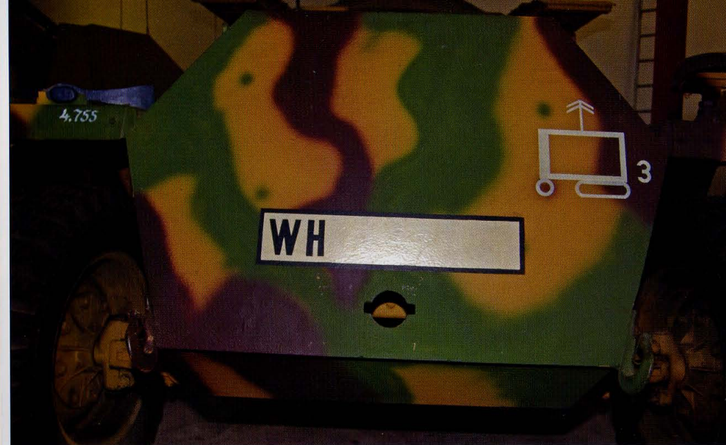
The front armor plate was 14.5 mm thick, and the circular aperture in the lower front of this armor plate was for the starting crank. A circular fairing covered this opening on most Ausf Ds. In fact during Wehrmacht operation, the circular covering was often deleted, and the last Ausf D production batches eliminated this cover at the assembly line.
