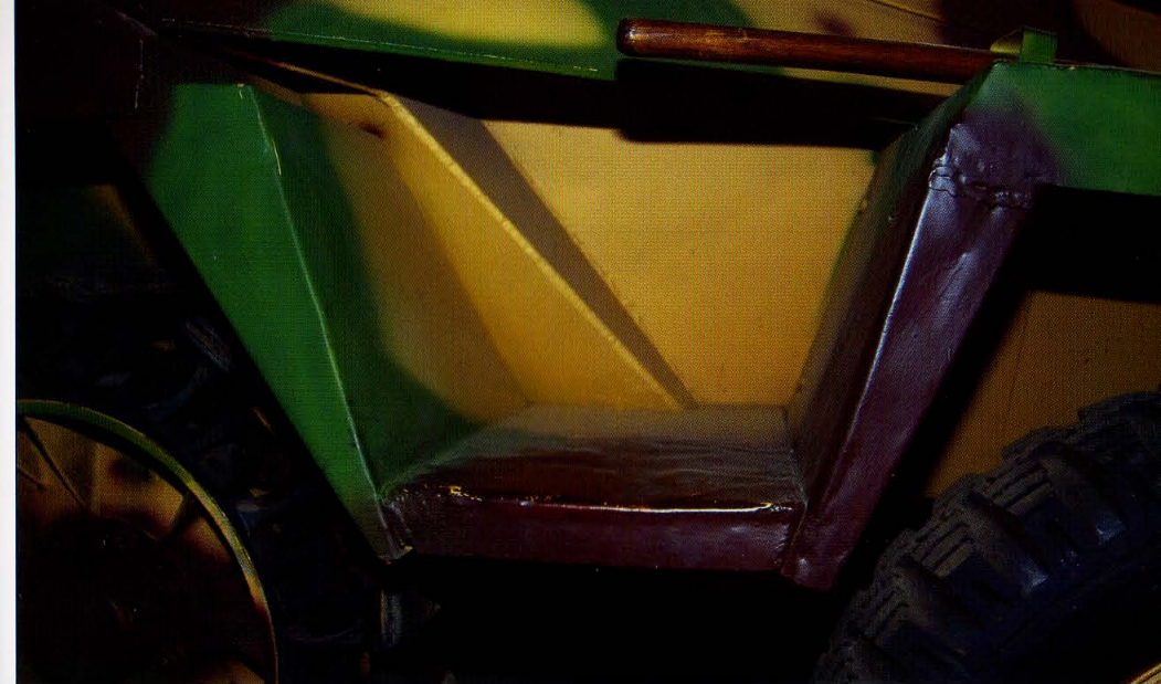
Compared to early Ausf Ds that adopted the Ausf C's front fender, the lower plate connecting the front fender with the track fender was longer on standard production Ausf Ds. Additionally, the shape of the forward slanted fairing was altered and became a triangular shape.
