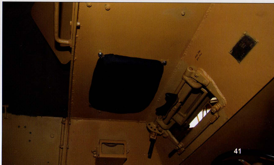
This view is of the left, armored roof. Only the driver and commander had an armored roof. A leather-covered cushion hangs from the roof. Just above the steering wheel is the visor. A small side visor is located on the inner side armor.
