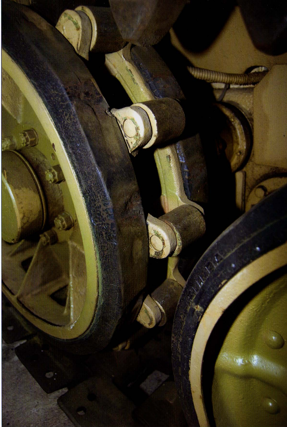
This drive sprocket is on the Ausf D's left side. A driving tooth on the inside of the track transferred power to the sprocket, which was equipped with rubber tires.
