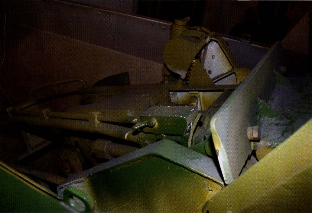
The small shield was attached on the upper portion of the barrel and moved with the gun. Left of the barrel is the elevation mechanism for the KwK 37 L/24 gun.
