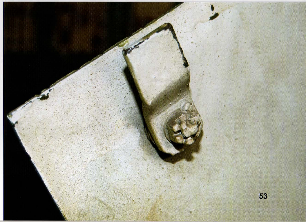
Early production German half-track vehicles lacked the rod-shaped opening mechanism that was a typical feature on standard production Ausf Ds. The rear doors could not be opened from inside, which made exiting through the rear doors impossible.
