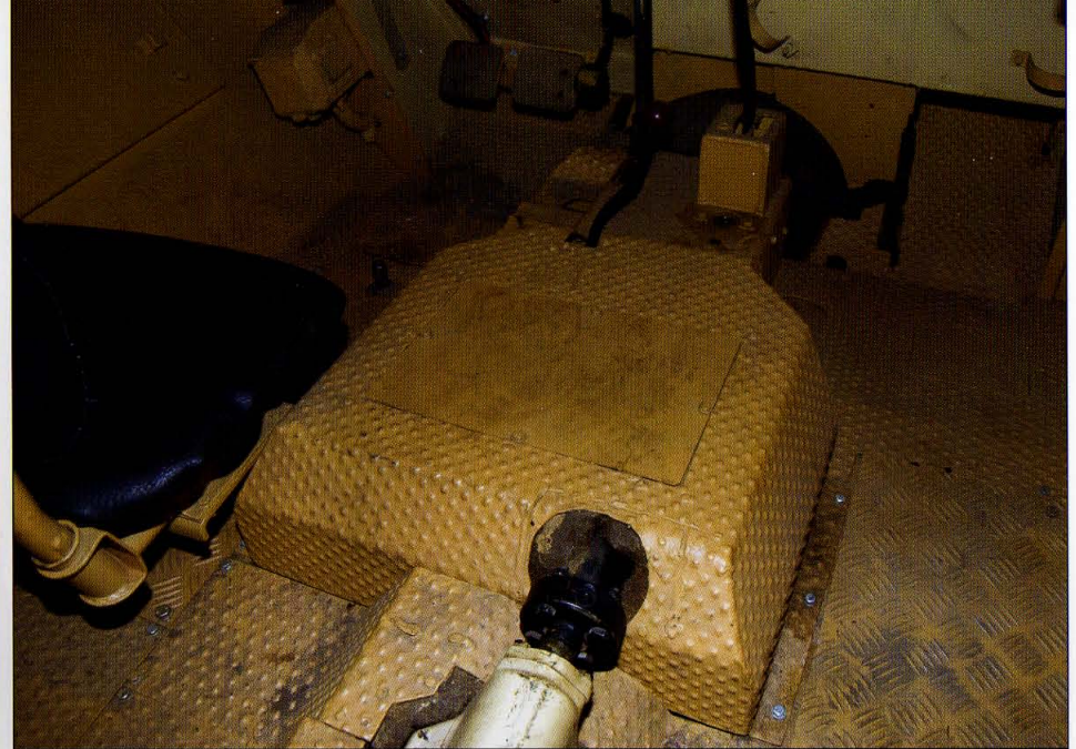
The fairing for the gearbox is located between the driver and the commander.
