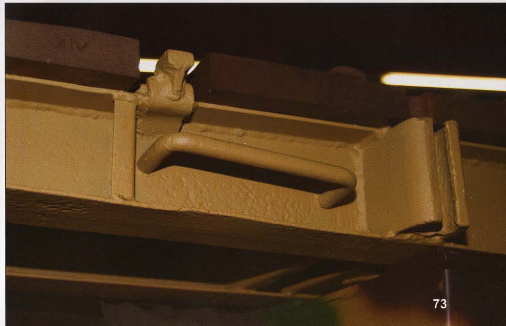
The rear arrangement of the right Übergangsschiene 8 rests on the support bracket. Note the circular aperture is located on the rear bracket.
