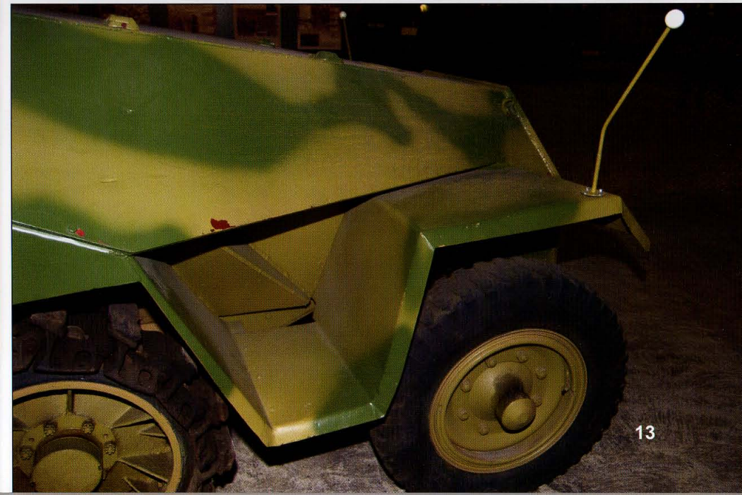
All Ausf Ds had no exhaust muffler on the vehicle's right side. So, only the left side had a muffler. The thickness of the fender's edge, which protected the tracks, is the same its entire length on this early production vehicle.
