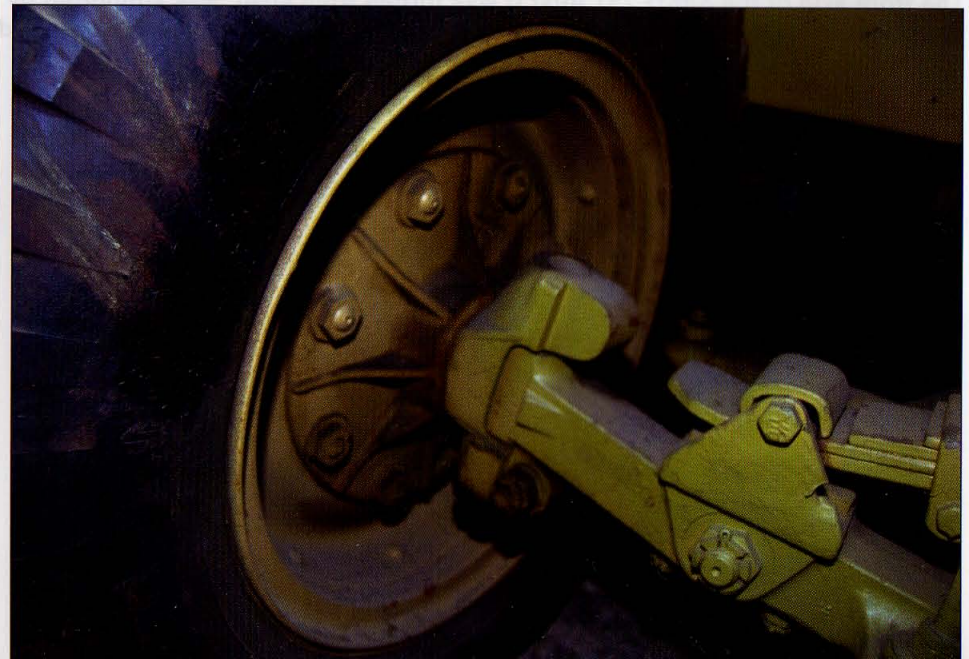
This right, front tire shot gives close-up access to the inner rim. The rims were made from pressed steel, and the right axis lacked a steering arm.
