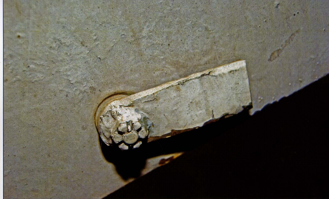
This view shows the left, rear entrance door's lower, inner fastener on a very early production Ausf D. Turning the upper and lower fasteners allowed the doors to open.
