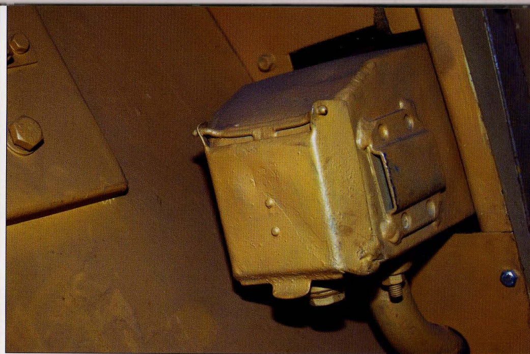
This device is a heater that thawed tubes connected to the cooling cycle of the engine and was a necessity for winter operation when temperatures could reach -30 degrees in areas where the Ausf D was stationed. The heater is located on the base of the left side armor. The curved tube below the heater directly leads to the engine compartment.
