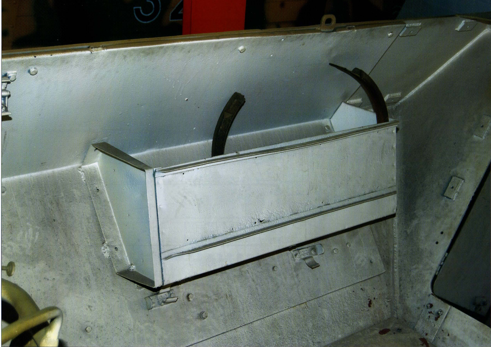
Instead of the headrest that was found on the SdKfz 251/1, the SdKfz 251/9 had a container located on the right inner surface of the vehicle's crew compartment.
