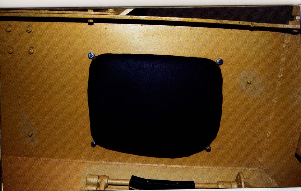
This cushion protected the commander's head. Leather covered this cushion, and screws secured it to the roof.
