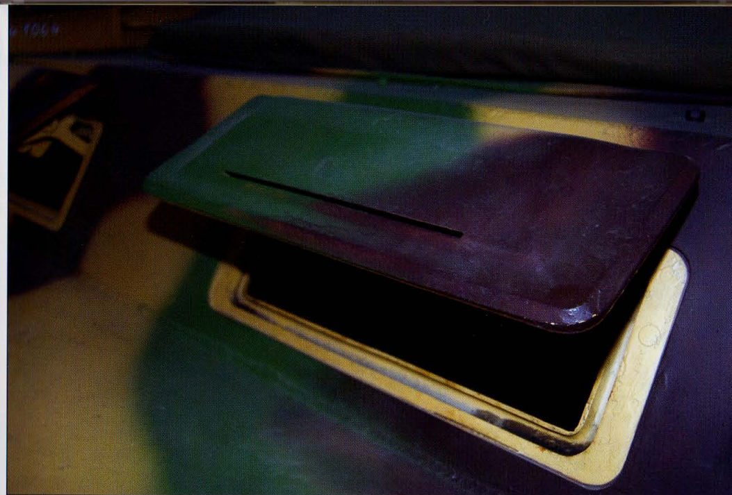
The armor plate for the left vision port had a slit cut into it. The left and right vision ports for the driver and commander, respectively, were identical.
