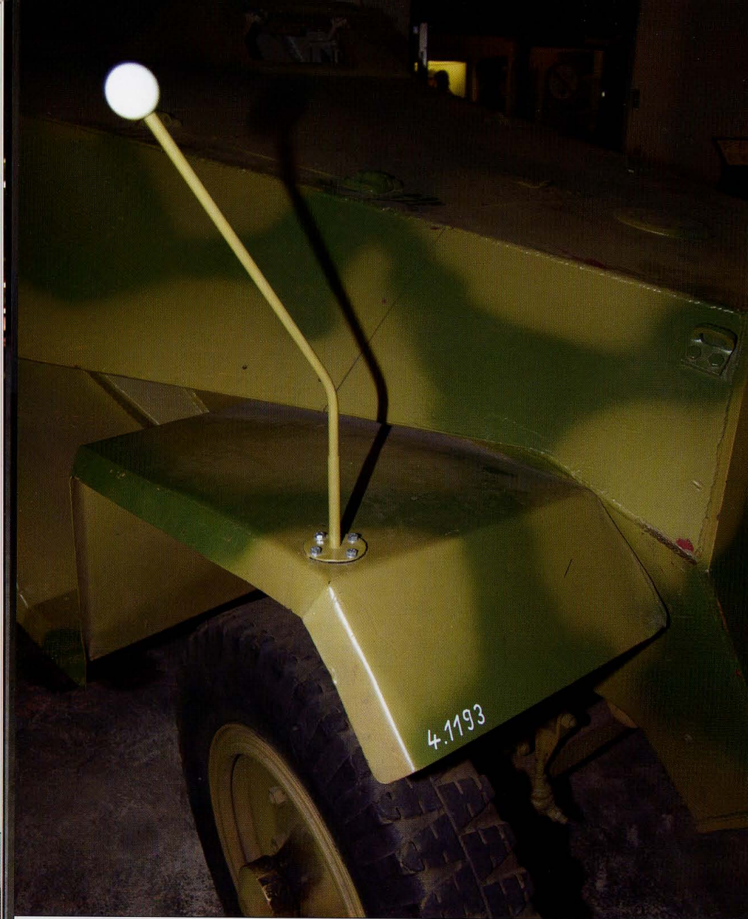
This rare, front-bent right fender indicates an early production SdKfz 251 Ausf D.
