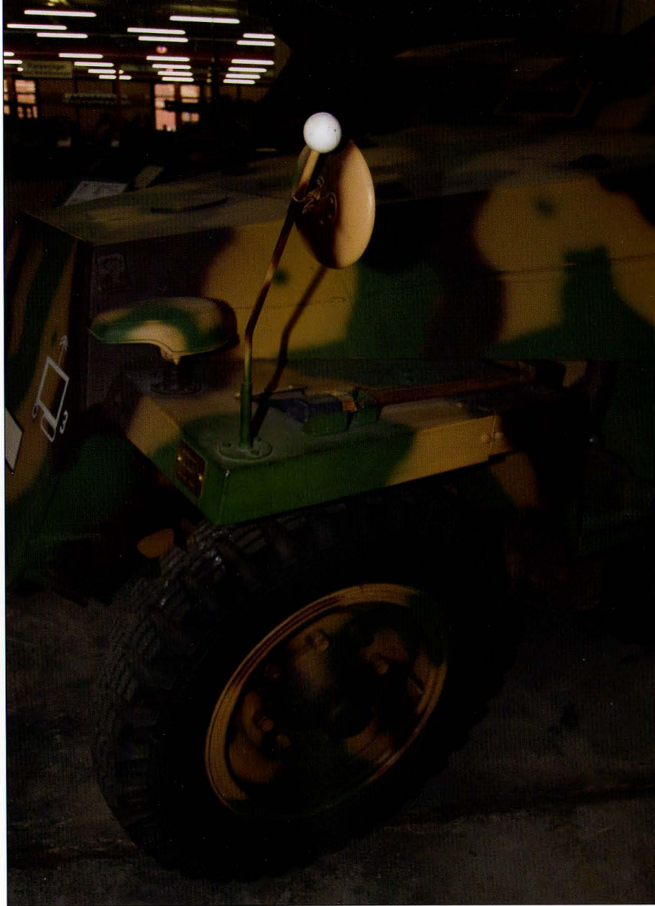
Two distinctive features for the majority of SdKfz 251 Ausf Ds was the straight fender design and a rear view mirror that was mounted only on the left boom to make vehicle production faster. While early production Ausf Ds had a position light mounted on the left and right fenders between the Notek blackout light and the boom, the standard production vehicle did not have these lights.
