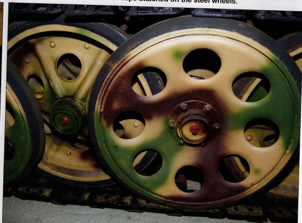
This view shows the tracked suspension of a late production SdKfz 251 Ausf D. These late vehicles had modified cover caps attached on the steel wheels.
