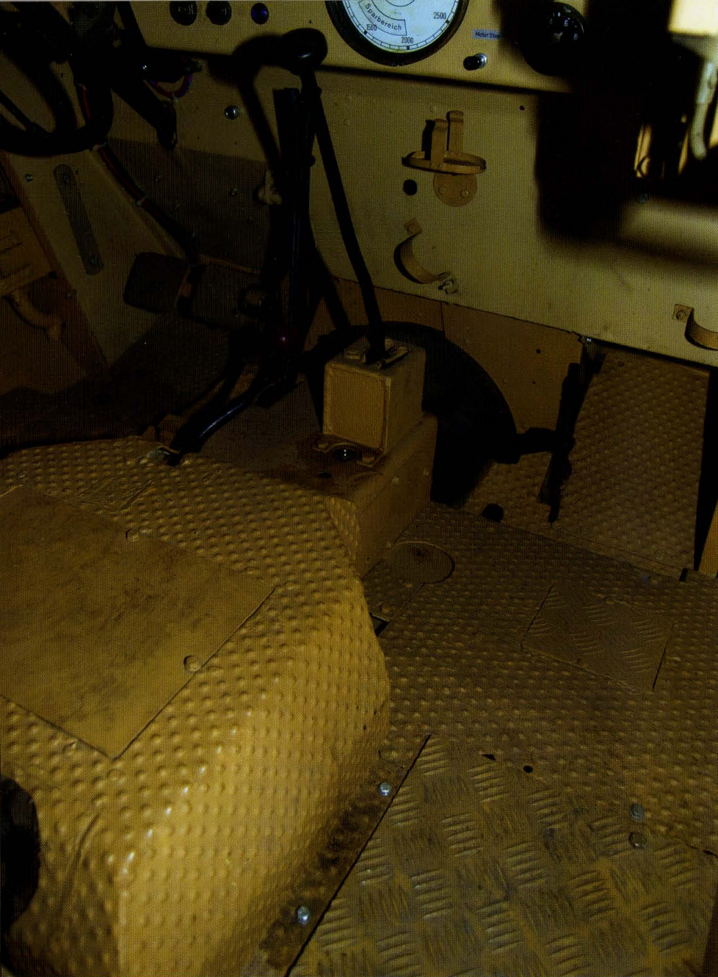
The gearbox and the engine reduction gearbox were covered by a fairing in the crew compartment. An access hatch is located on top of this covering.
