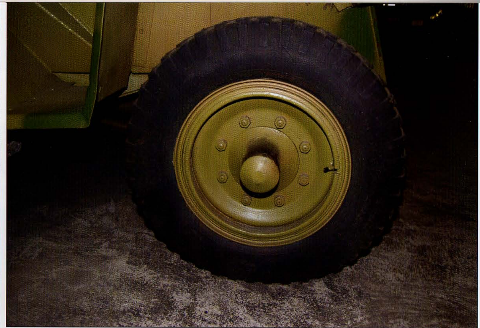
This view highlights the right-side front tire and its rim. The front wheels were 575 mm in diameter and had no brake system. The tires consisted of synthetic rubber called Buna, which used brown coal as its base. Beginning in 1937, the IG Farbenindustrie AG produced Buna in large quantities since the Third Reich did not have access to natural rubber from the Far East.
