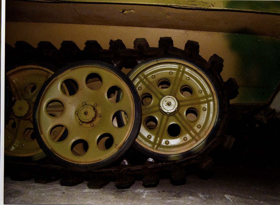
The rear idler tensioned the track. The rubber-tired idler wheel has a diameter of 575 mm and is attached on a crank arm that is sprung by a torsion bar.
