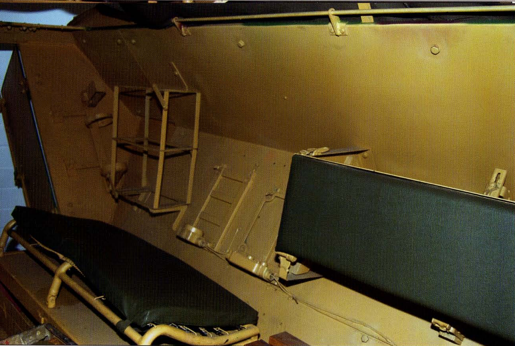
Typical SdKfz 251/7 engineer vehicles had a frame attached to the rear, on the left side of the crew compartment. Standard production SdKfz 251/1s did not have this frame.
